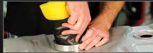
Insert foam inside the tank
