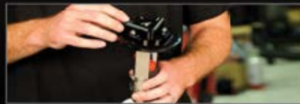
Install c-ring, pump, and tighten nuts
