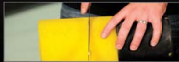
Cut hanger 1 in SHORTER than tank depth
