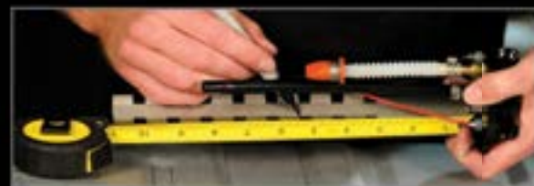
Cut hanger 1 in SHORTER than tank depth
